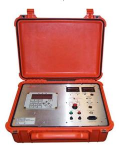
Alternative kits are now available with <1° resolution torque & angle transducer, T-Box XL based tool controller with torque & angle display / capture / storage, & visual rotation indicator. Please contact Norbar for more information.
